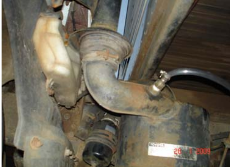
Hydroxy line feed into the air filter box
