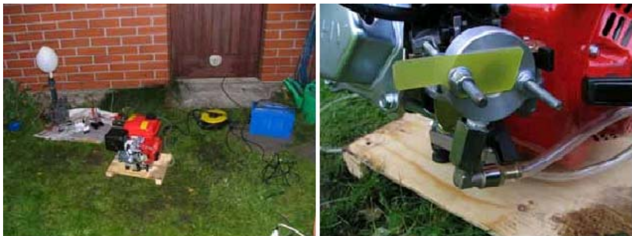
Figure 14. 6.5hp 200cc 4-stroke running on electrolytic gas
