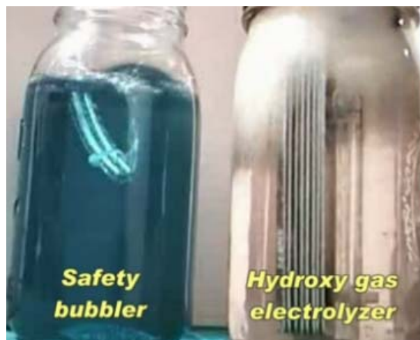
Pictured in the right container are stainless steel plates used as electrodes, above them is
