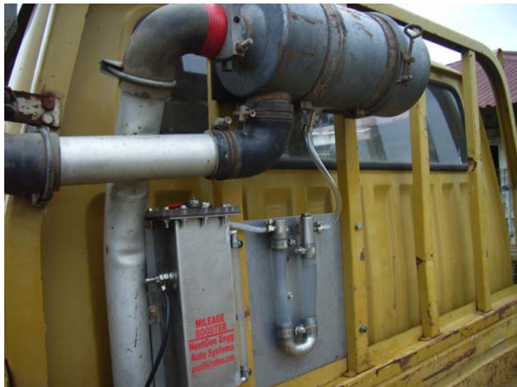
Panacea's diesel installation using Praveen's open source booster
